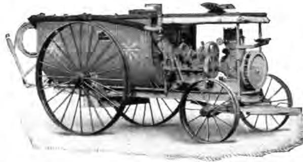
**BEAN Giant Triplex No. 748** with 6 H. P. BEAN engine and BEAN Giant Triplex Pump. Capacity 12 gals. a minute at 300 lbs. pressure. Turn-under truck and flexible coupling.
