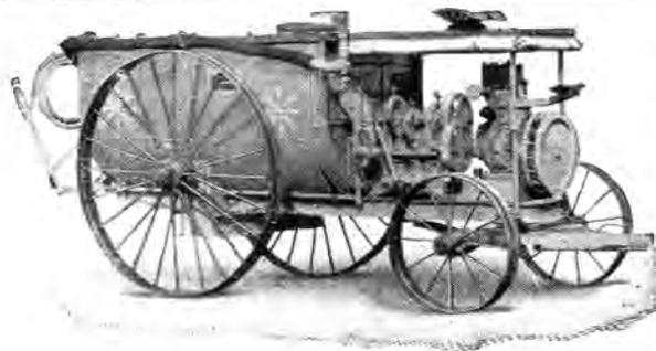
BEAN Giant Triplex No. 748 with 6 H. P. BEAN engine and BEAN Giant Triplex Pump. Capacity 12 gals. a minute at 300 lbs. pressure. Turn-under truck and flexible coupling.
