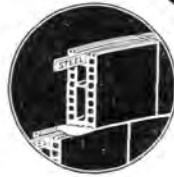
Nasco Silo Wall. Note perforated shell, providing firm anchorage for mortar joints.
