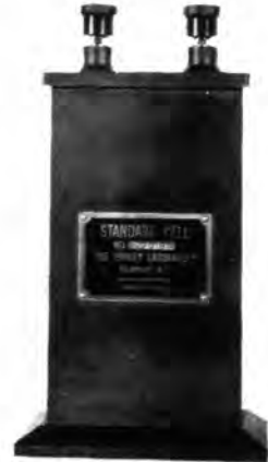
This little box of magic is the "standard of standards" which helps to insure the hair-splitting accuracy of electric meters.
