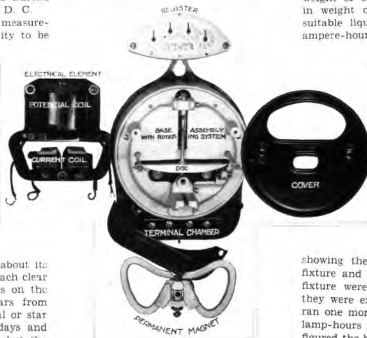
This is what the "destroying angel" found when the meter was taken apart to see what made it go.
