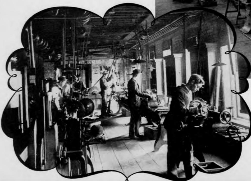
*Left:* Students working on iron lathes in the mechanical laboratory, about 1893. See overhead belts and pulleys. *Above:* In shops such as this, mechanical engineering students study industrial production.
